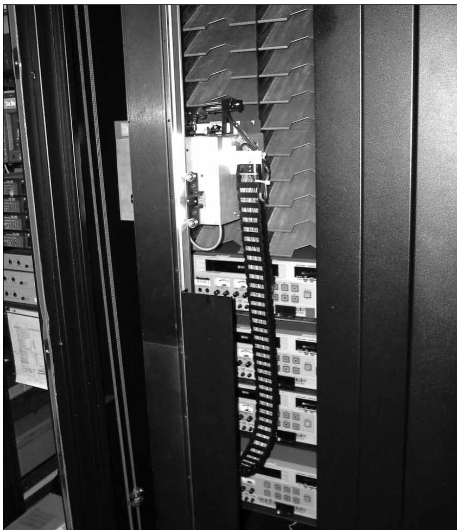
FIGURE 4. This tape robot was used to digitize archival content.
