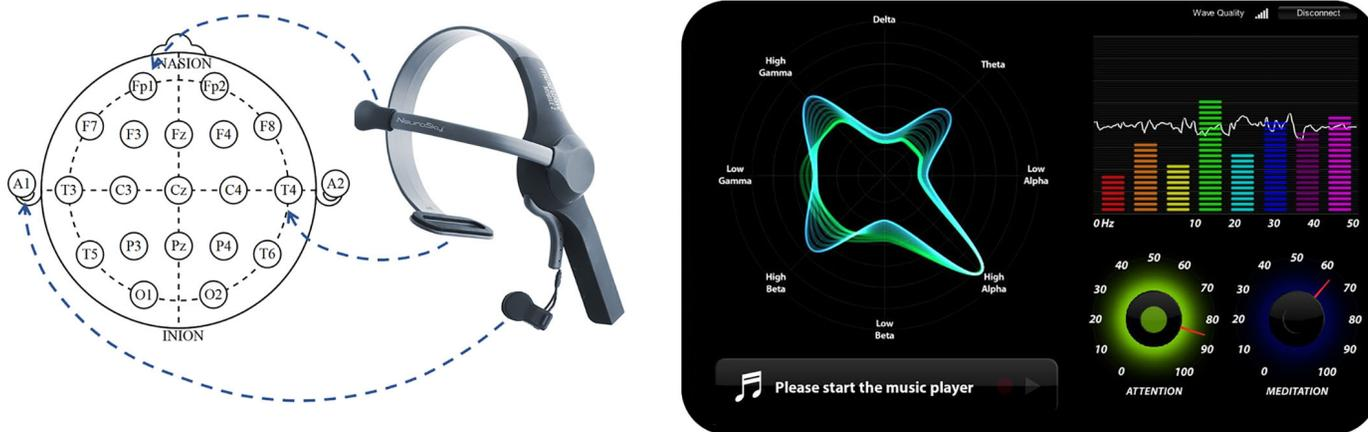
**Figure 1.** (Left) NeuroSky MindWave headset. (Right) NeuroSky demonstration software.
