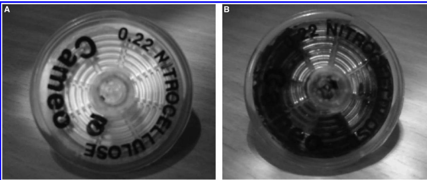
**Figure 4.** Images of the filters (A) before and (B) after “smoking.”
