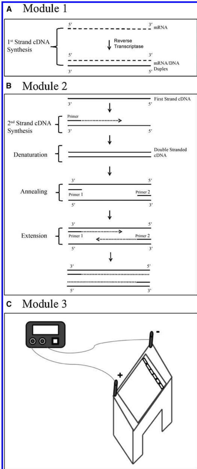
**Figure 1.** Schematic diagram of experiments used in each module. (A) Module 1: preparation of cDNA using reverse transcriptase. (B) Module 2: amplification of gene-specific cDNA using PCR. (C) Module 3: agarose gel electrophoresis of PCR products.
