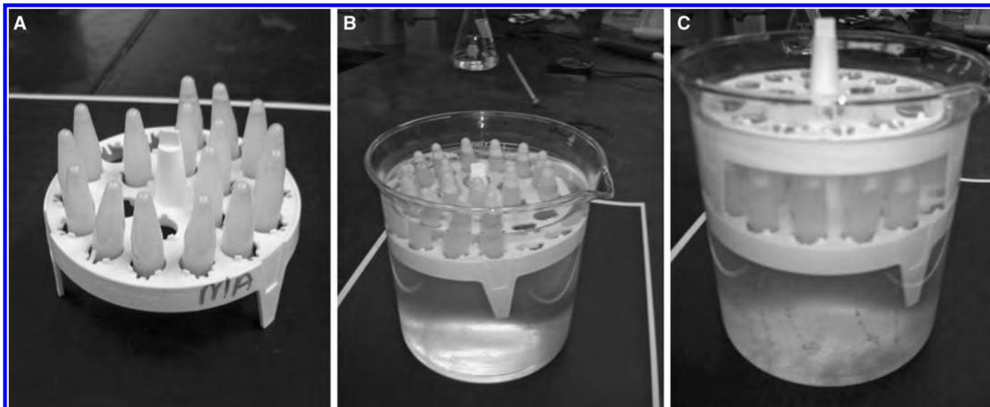
**Figure 1.** Assay setup. (A) Microcentrifuge tubes inverted into rack. (B) Rack placed into beaker with 40°C water. (C) Rack lowered into water by placing empty rack on top to completely submerge the tubes. Yeast–glucose mixture can be seen entering the water bath.
