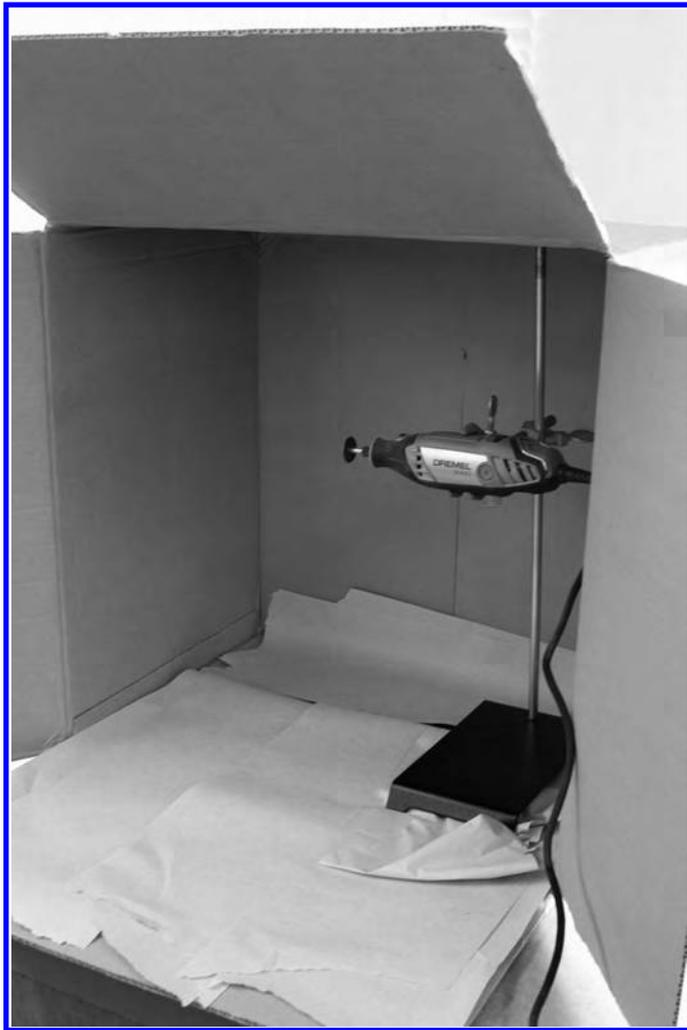
**Figure 4.** Picture of the setup for the ex ovo preparation.
