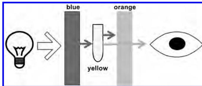
**Figure 2.** The tubes (yellow) are excited by blue light obtained by placing a filter between the light source and the sample. The fluorescent light is observed by having an orange filter between the sample and the observer.
