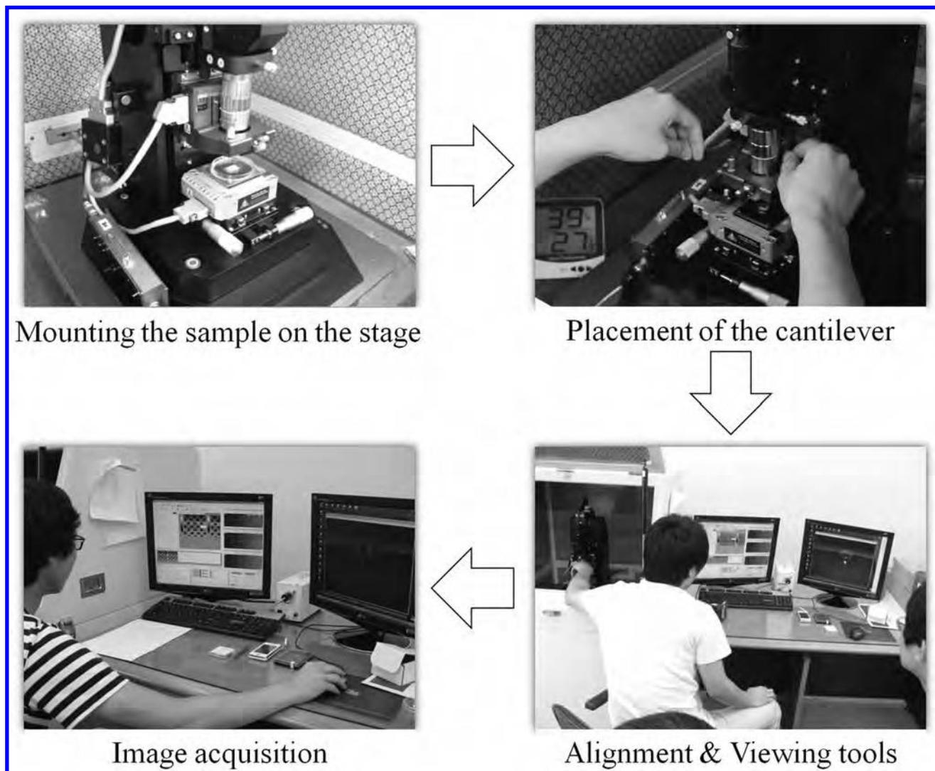
**Figure 4.** AFM system operation.
