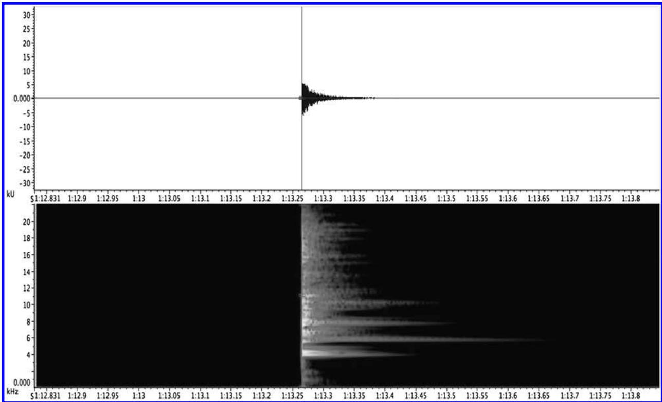
**Figure 2.** Two ways in which students can visualize underwater acoustic data of a single snap from a shrimp (*Synalpheus heeia*) using the software Raven Lite 1.0 (Chaif et al., 2006). The top image displays the data as a waveform (amplitude measured in kU vs. time). According to the data, this snap had a peak intensity of ~6 kU and the snap had a duration of ~0.2 seconds. The bottom image displays the same snap in the form of a spectral frequency (frequency in kHz vs. time).
