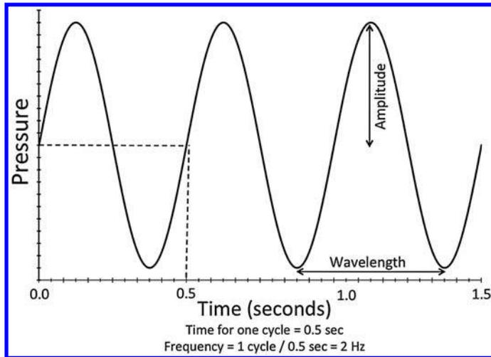
**Figure 1.** A sound wave as a sinusoidal graph of pressure versus time, showing the wave's basic components: frequency, wavelength, and amplitude.
