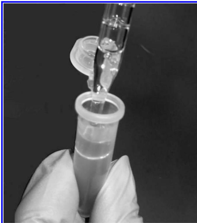
**Figure 5.** Applying oil to MEEP surface.
