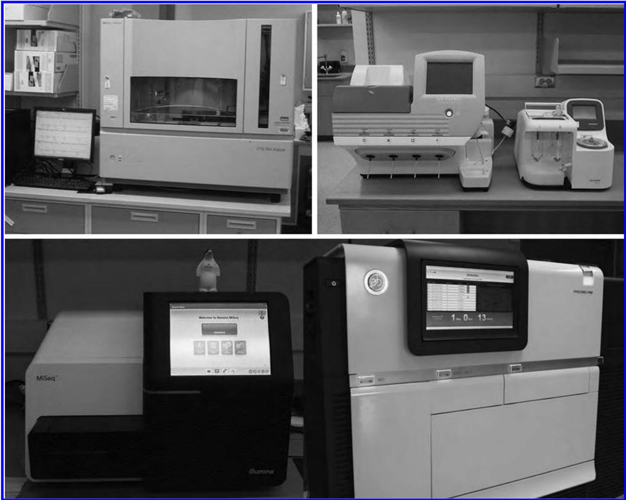
**Figure 1.** An Applied Biosystems 3730, Life Technologies Ion PGM, Illumina MiSeq, and Pacific Biosciences PacBio RS instruments. Image of the PacBio RS courtesy of <http://gqinnovationcenter.com/services/sequencing/technoPacBio.aspx?l=e>.
