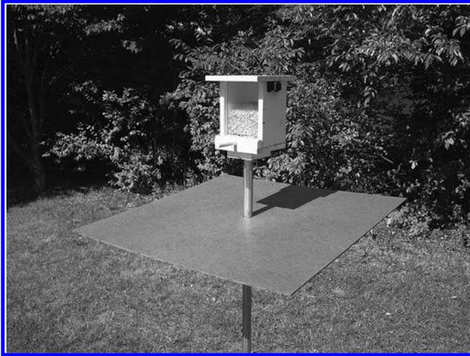
**Figure 1.** One of the bird feeders used in the experiments. The feeders are made from PVC, have oak-dowel perches, and sit atop poles made from electrical conduit. The dark object below the feeder lid is a magnetic catch.
