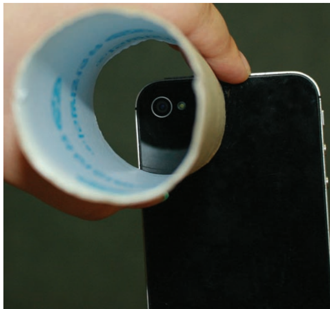
Figure 4. Alignment of the adaptor tube with the cell phone camera.
