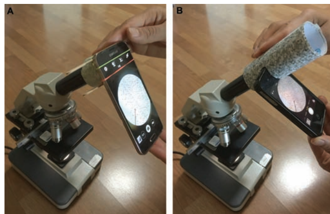
Figure 6. CellCam mounted on a microscope, showing proper alignment of image: (A) mid-mounted camera version; (B) corner-mounted camera version.
