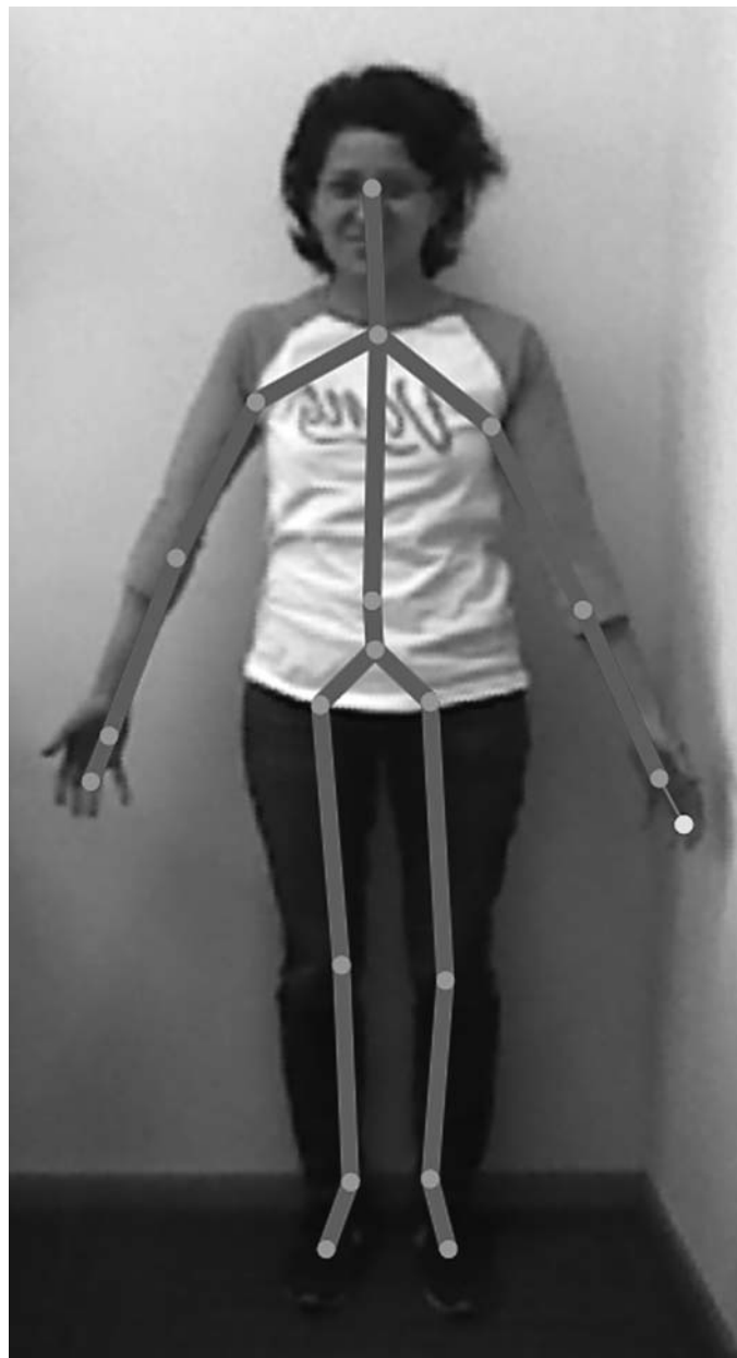
Figure 2. Combination of depth data and color data. The green points represents the joints of the body.
