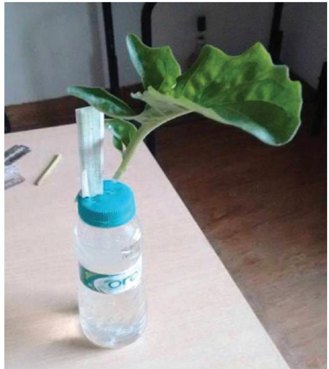
**Figure 2.** Operation of the single-leaf potometer with water.
