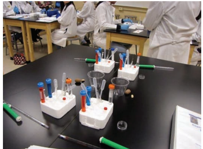
Figure 6. Lab set-up for alginate lab. Each styrofoam test tube holder contains a tube of 0.5% (not shown), 1.0% (red) and 2.0% (blue) solutions of liquid sodium alginate, a tube of calcium chloride solution, 3 plastic pipettes of different diameter openings, needleless syringe, pair of forceps, 10 mL plastic pipette with pipette pump to transfer calcium chloride, cup of rinse water, small Petri dish per student, small capped vial per student, a pecan (size of human ovary), and pistachio (size of rhesus monkey ovary).
