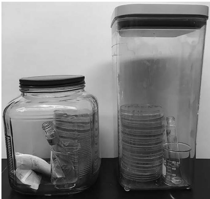
**Figure 1.** Low-cost anaerobic chamber system. (Left) Anaerobic chamber using Cracker Jar (glass), 3.8L. (Right) Anaerobic chamber using OXO Pop Container, 5.5L, Airtight Seal. Petri plates, anaerobic indicator, and Hot Hands packets are visible in the Cracker Jar (glass container). HotHand packets are present in the OXO Pop Container on the right, but have been moved behind the petri plates to better show the anaerobic indicator.
