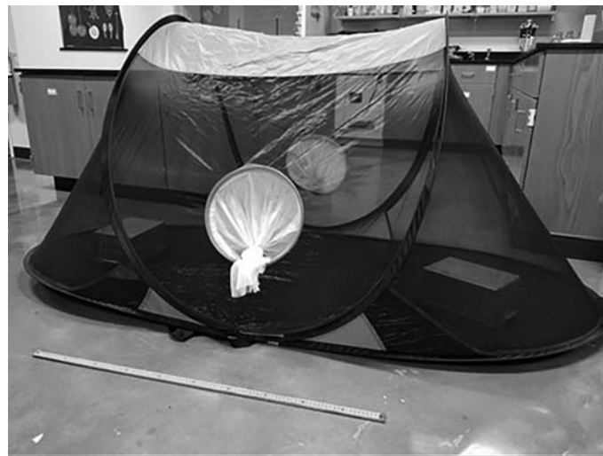
Figure 3. The insect-proof tent is a collapsible one-person tent modified with two mesh-lined sleeves for controlled access. Students add and remove traps through the sleeves without releasing flies. Photo credit: Alison Onstine.
