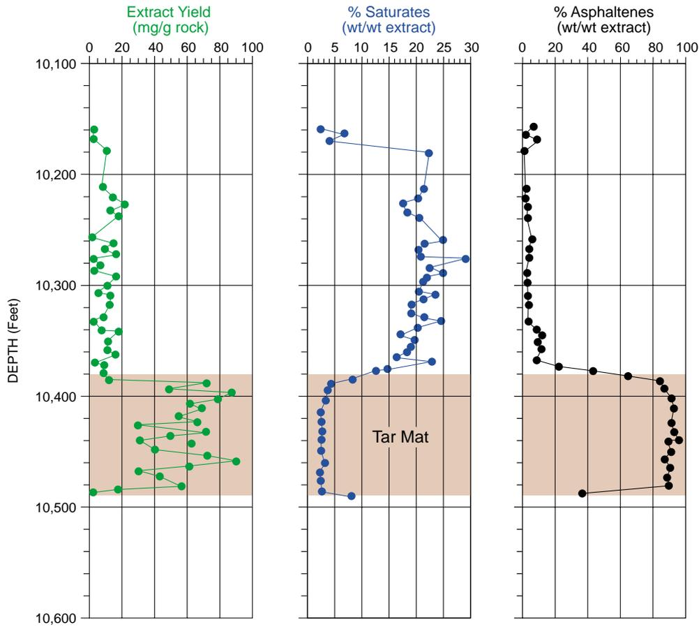
Figure 6: Well-C: extract yield, and proportions of saturates and asphaltenes versus depth.
