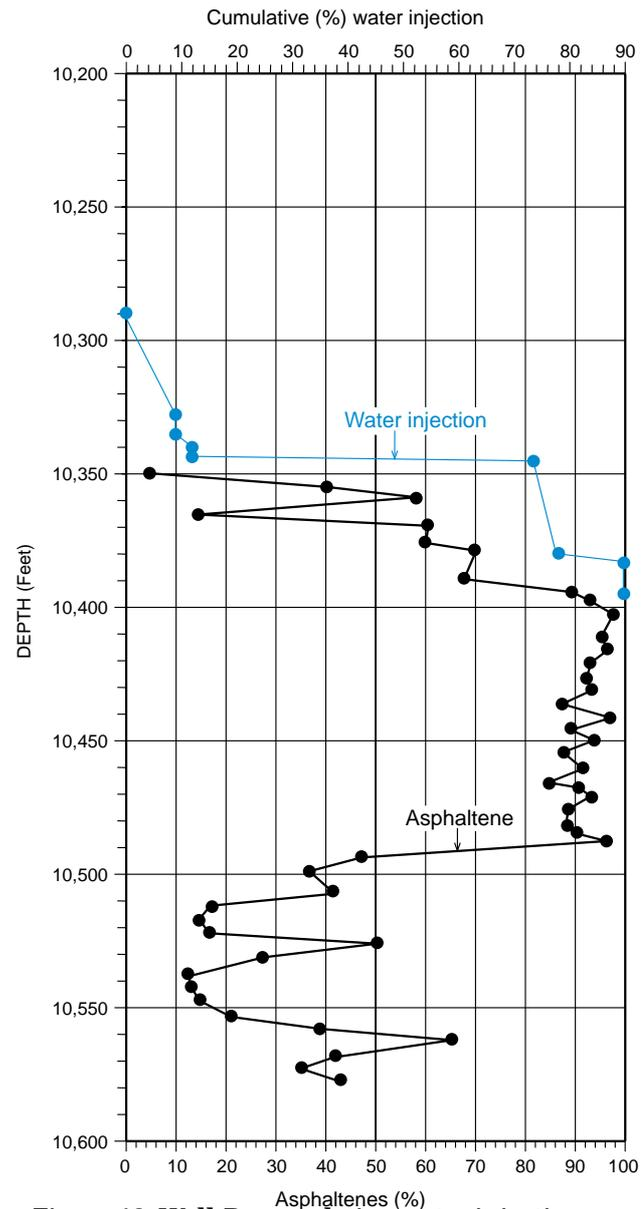
**Figure 18: Well-B: cumulative water injection versus asphaltene content.**
