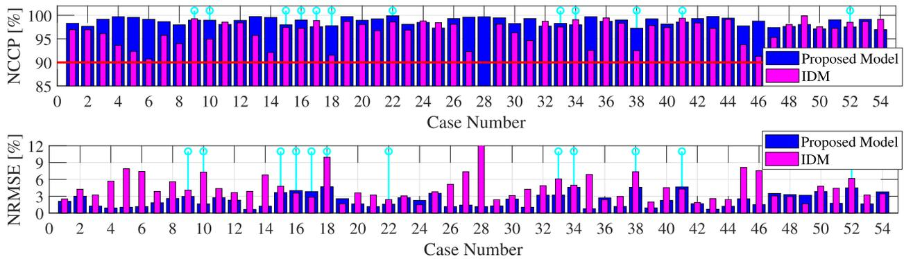
**Fig. 5** NCCP and NRMSE of the proposed model (blue bar) and IDM (magenta bar) for 54 braking-to-stop cases. Vertical cyan lines represent for car-following situations.
