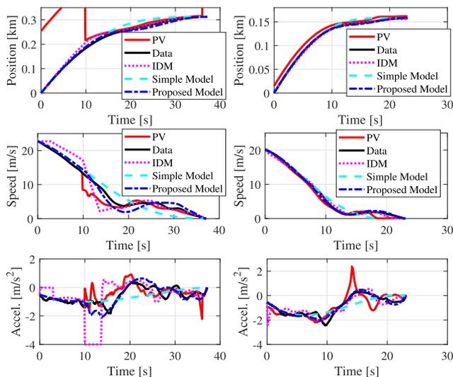
**Fig. 6** Comparison of state trajectories between models and data in case numbers 18 (left) and 22 (right). PV is the preceding vehicle, and the simple model is the model using only type 1 solution that cannot describe the car-following feature.
