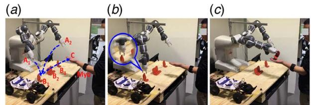
**Fig. 1 The robot collaborates with its human partner for assembling a high-fidelity model vehicle: (a) before picking up, (b) picking up, and (c) delivering**
