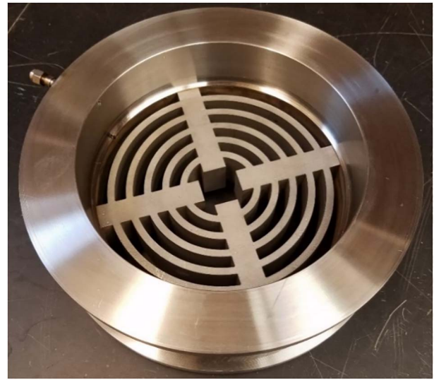
Fig. 9 Refined hot heat exchanger design
