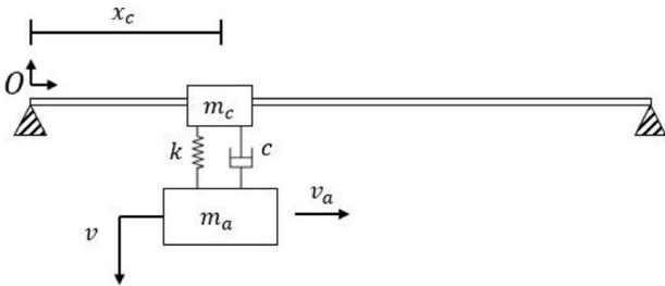
**Fig. 3** Schematic of the mobile damping robot on the cable
