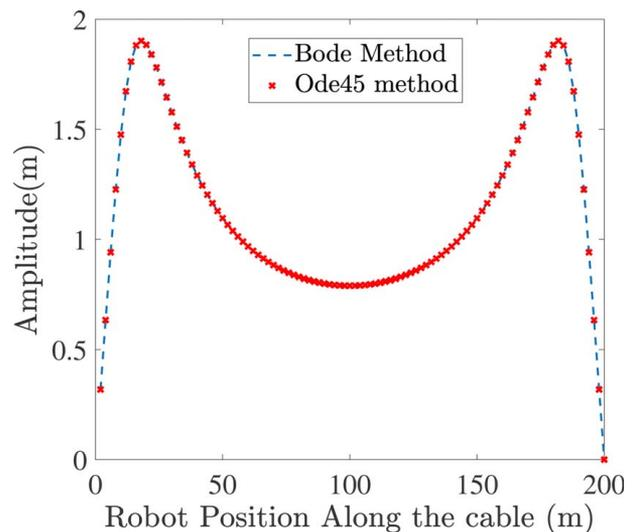
**Fig. 4 Model validation by comparing the response of the cable-robot system using two methods: ODE45 and bode. The cable is excited by a uniformly distributed wind force.**
