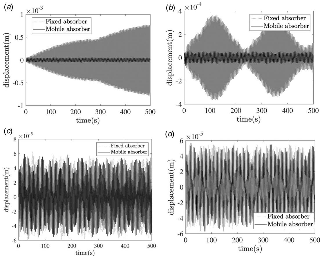
**Fig. 7 Comparison of a fixed damper and the mobile damping robot for  $w_{10} = 3$  Hz: (a) at node, (b) 10% away from node, (c) 30% away from antinode, and (d) at antinode**
