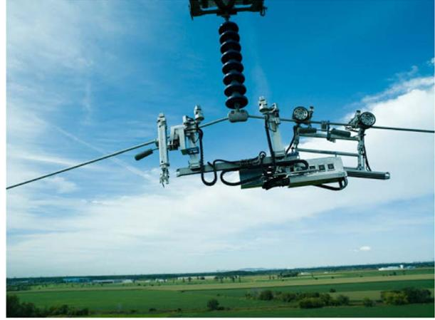
**Fig. 1** Presentation of a FPVA and an inspection robot: (a) stockbridge damper and (b) Hydro-Quebec lineScout inspection robot
