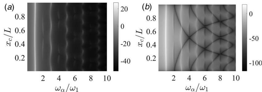
Fig. 6 Frequency response of the cable and the robot along the span: (a) normalized cable frequency response along the span and (b) normalized mobile damping robot frequency response along the span
