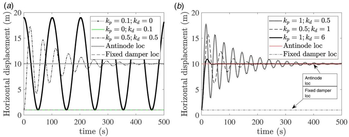
Fig. 5 Comparing the values of  $k_p$  and  $k_d$  for optimal control
