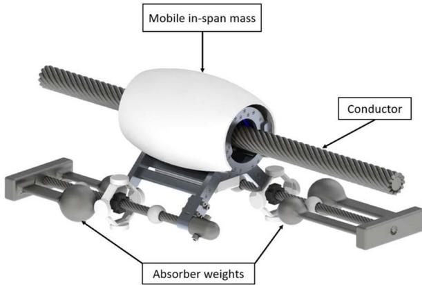
**Fig. 2** Conceptual design of the mobile damping robot attached to a conductor
