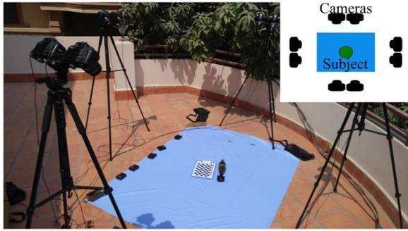
**Fig. 1** This figure shows the configuration of the eight-camera image acquisition setup. Each of the cameras is zoomed and focused on the piece of ordnance and checkerboard (used as a reference for scale). The diagram in the bottom right of the figure shows the relative positions of the cameras, as some are difficult to distinguish from the foliage in the background.
