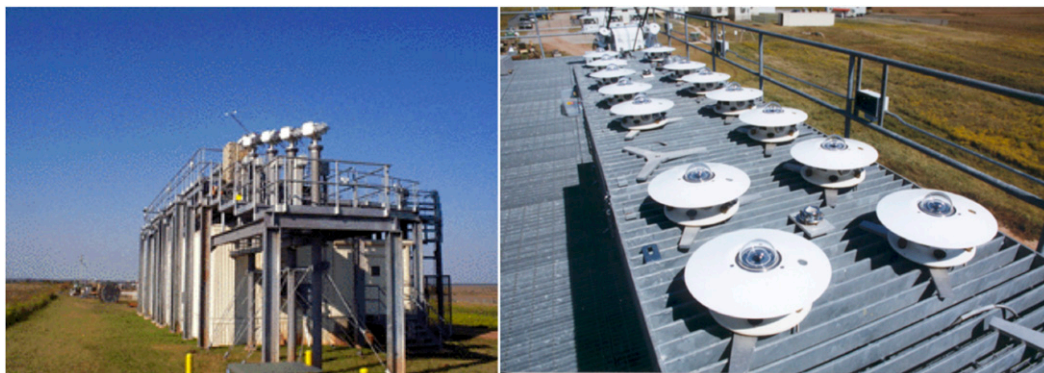
FIG. 16-1. The Radiometric Calibration Facility at the ARM Southern Great Plains site near Billings, Oklahoma; close-up of pyranometers being calibrated at the facility.
