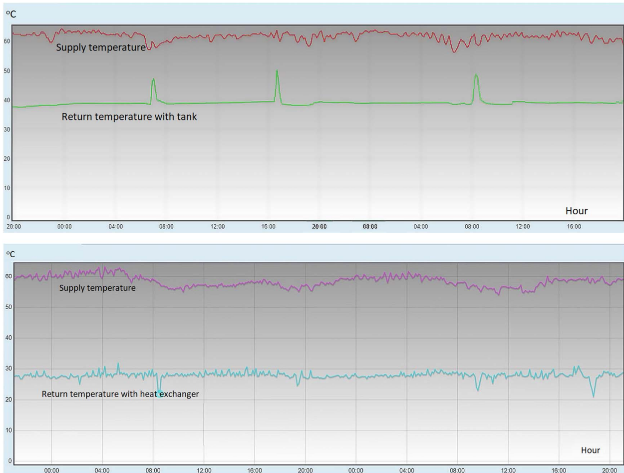
Fig. 4 Temperatures in one of the houses before and after replacing the hot water tanks with instantaneous heat exchangers. The upper diagram shows measurements on August 16–17 in house 3 before the replacement. As seen, the return temperature is in general as high as 40 °C (green curve), and when hot water is consumed the return rises to 50 °C. The lower diagram shows measurements of the same house on November 8–9 after the replacement (magenta curve). As seen, the return is now below 30 °C and when domestic hot water is tapped it is even close to 20 °C.
