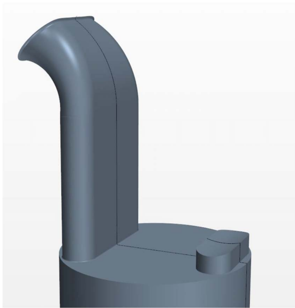
Fig. 8 CAD geometry, rotary valve cylinder head in intake configuration
