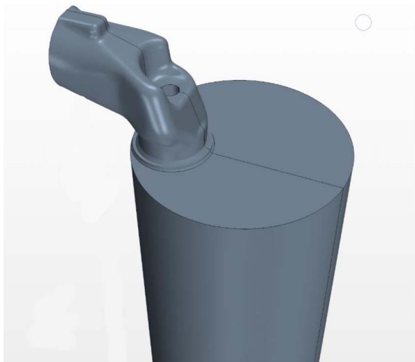
Fig. 5 CAD geometry, poppet valve cylinder head in exhaust configuration
