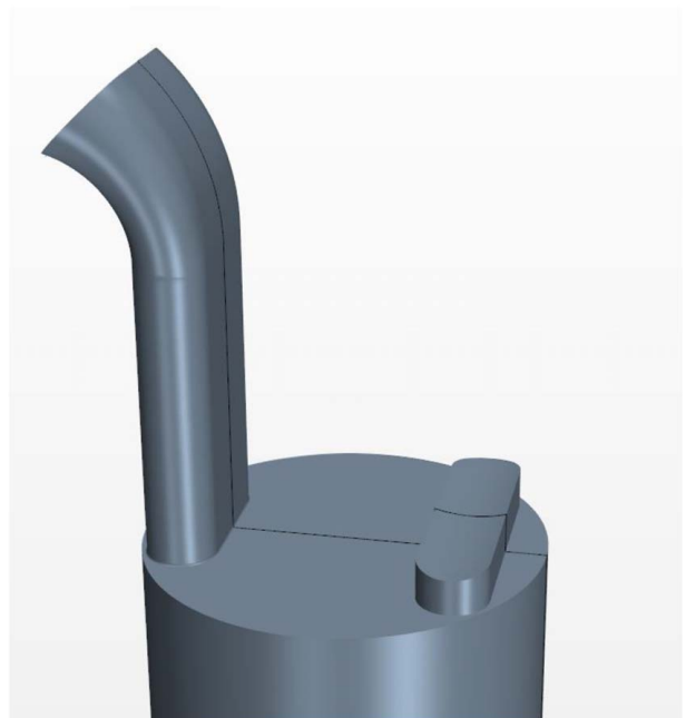
Fig. 7 CAD geometry, rotary valve cylinder head in exhaust configuration
