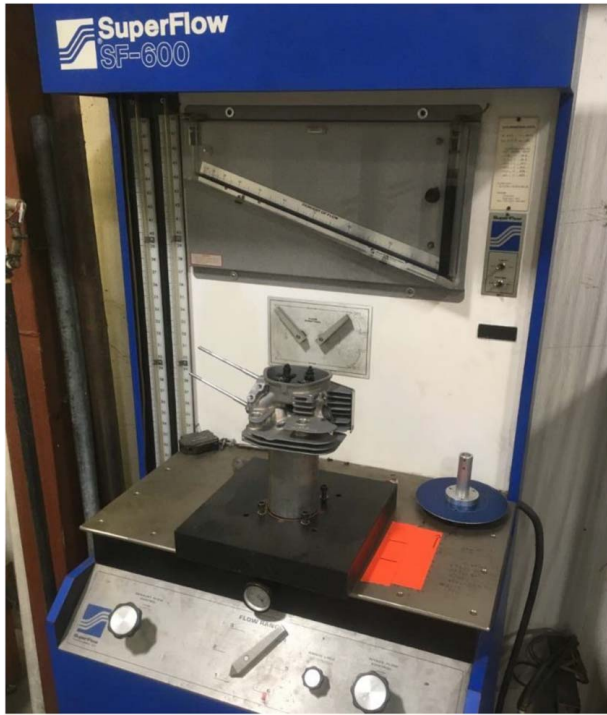
Fig. 4 SF-600 flow bench with poppet valve cylinder head
