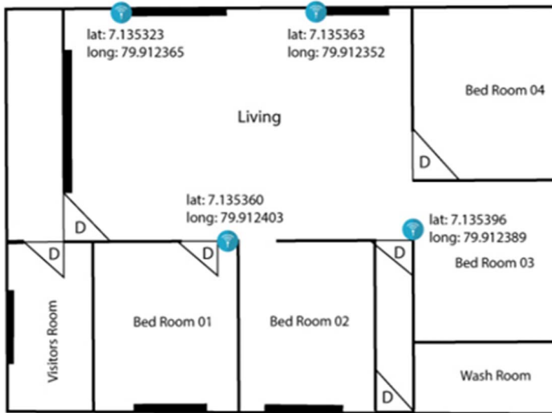
Fig. 4 Beacon deployment in the experimental area
