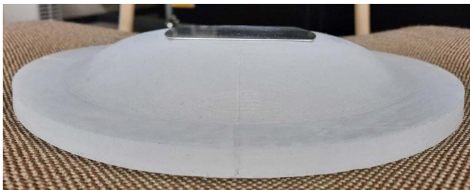
Fig. 4 Developed system, metallic box coupled with a silicone rubber 80 shoreA disc
