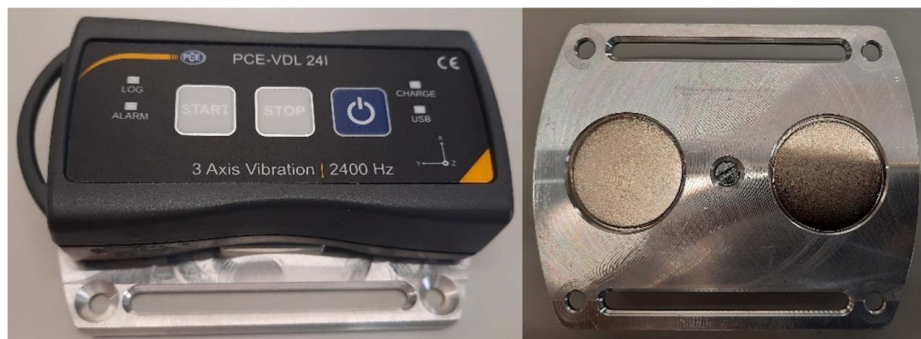
Fig. 1 Three-axial accelerometer attached on the mounting plate
