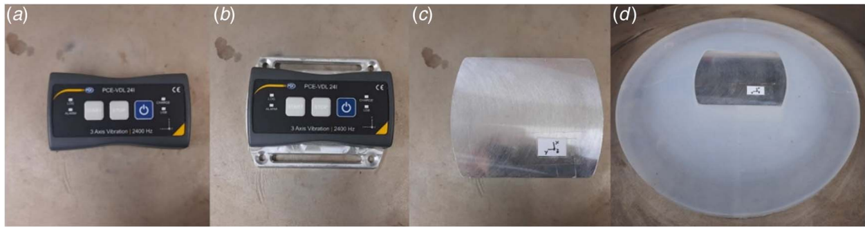
Fig. 5 Experiments examples and axis configuration: (a) accelerometer, (b) mounting plate, (c) metallic box, and (d) rubber disc/full equipment
