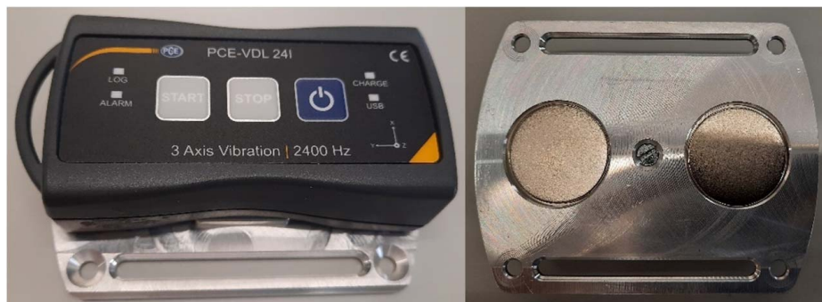
Fig. 1 Three-axial accelerometer attached on the mounting plate
