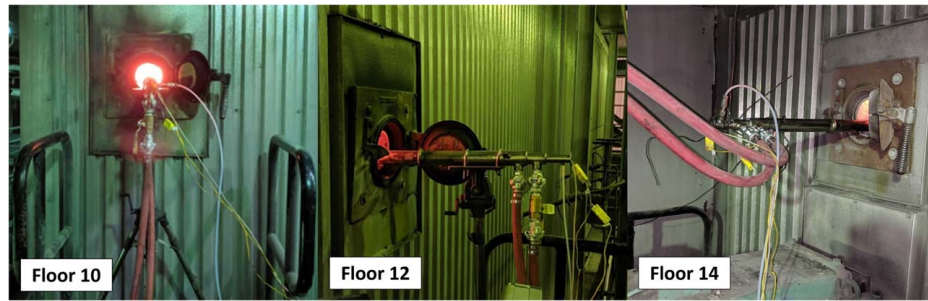
Fig. 1 Images of University of Utah narrow-angle radiometer setup at each boiler elevation examined
