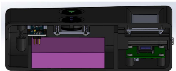
Fig. 12 Final design of handheld harmful algae monitoring device
