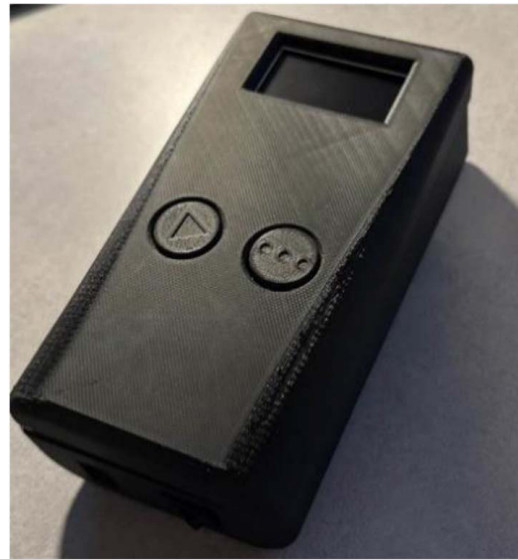
Fig. 14 3D printed final design of handheld harmful algae monitoring device
