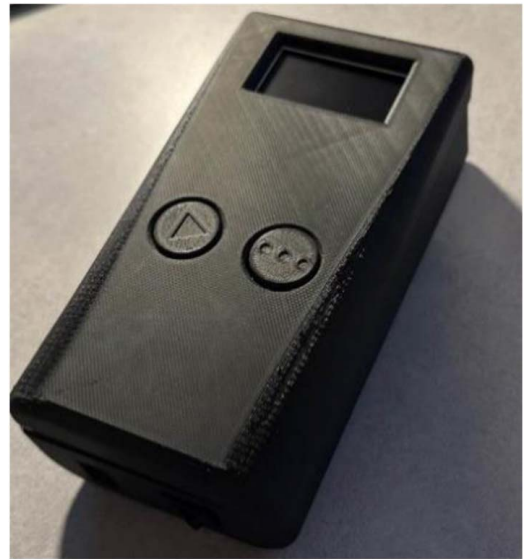
Fig. 14 3D printed final design of handheld harmful algae monitoring device
