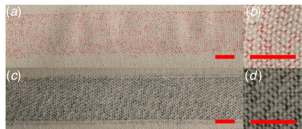
Fig. 3 Back of uncovered peel samples created with a bed temperature of 100 °C after part is created on fabric: (a) Type 1 fabric sample; scale bar is 10 mm, (b) close up of Type 1 sample, (c) Type 2 fabric sample, and (d) close up of Type 2 sample
