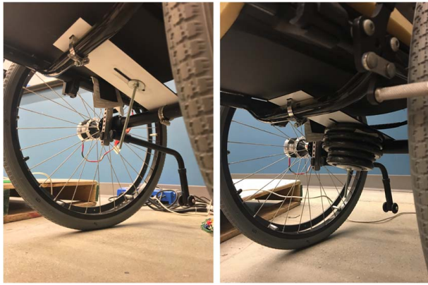
Fig. 2 (Left) Unloaded platform to support up to 4 kg of added mass to the drive wheel axle. (Right) Axle platform loaded with 4 kg of weight plates.
