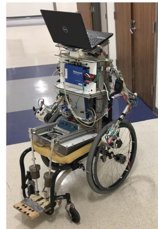
Fig. 1 The robotic wheelchair-propelling anatomical model propulsion system seated in the Quickie GT wheelchair
