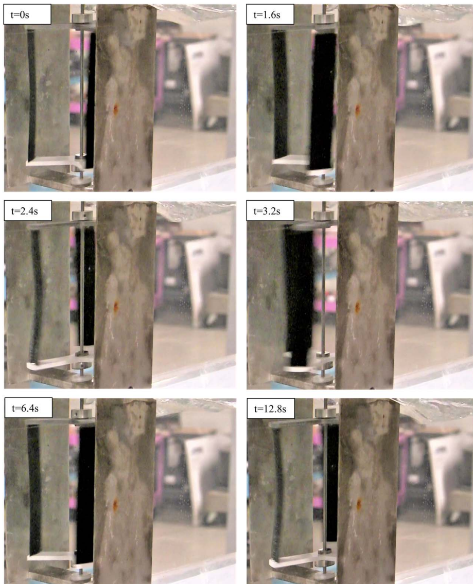
Fig. 7 Instantaneous images of flexible (75–85 Shore A hardness) blade turbine at a flow speed of 0.68 m/s while operating
