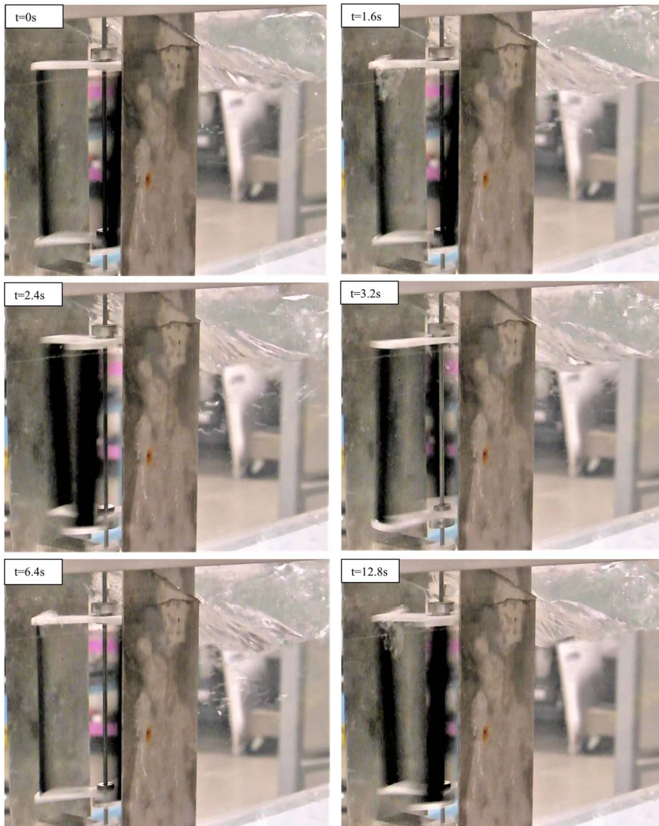
Fig. 8 Images of a less flexible (85–95 Shore A hardness) blade turbine at 0.68 m/s flow speed while operating
