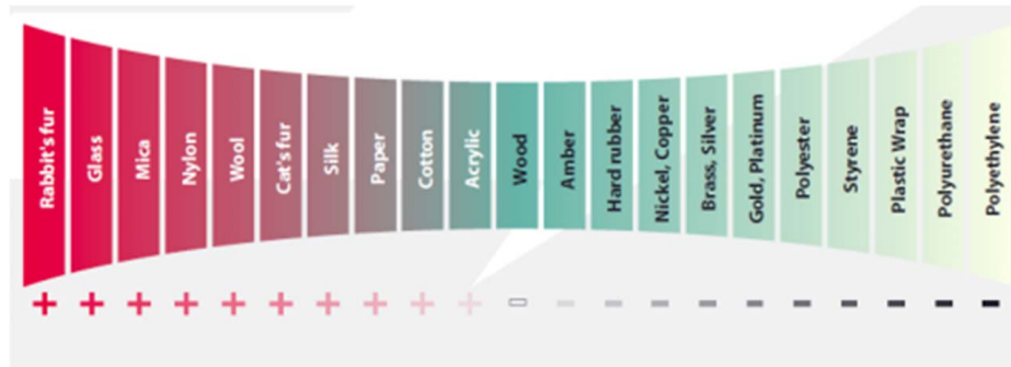
Fig. 1 Typical triboelectric scale: materials on the left side tend to be positively charged, whereas materials on the right side tend to be more negatively charged 6 (with permission from EXAIR LLC, 11510 Goldcoast Drive, Cincinnati, Ohio 45249-1621)
