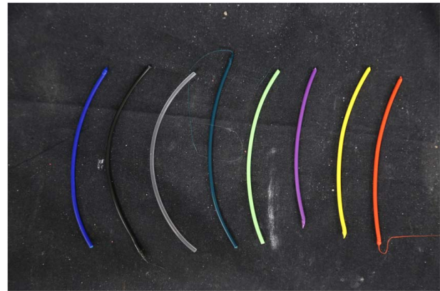
Fig. 1 Eight filament sections corresponding to tested filament colors
