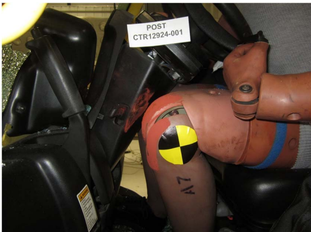
Fig. 4 ATD Knee contact with steering column in barrier test
