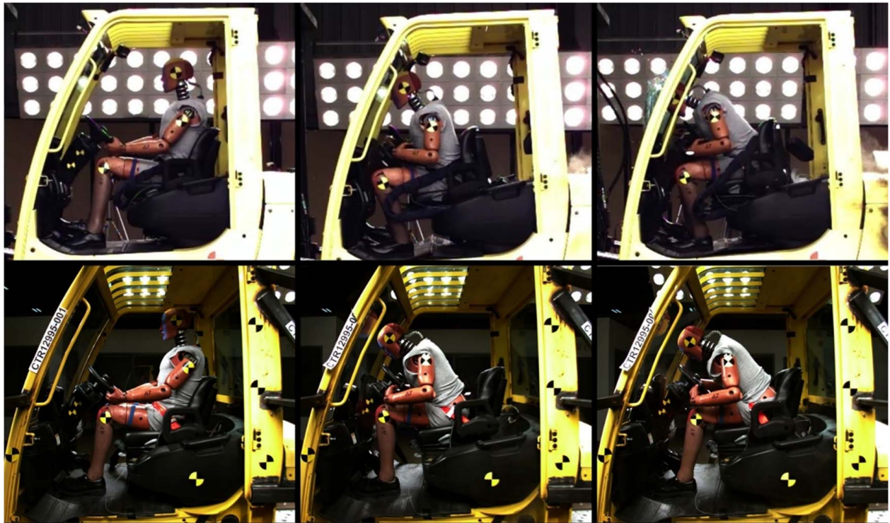
Fig. 6 Comparison of ATD kinematics at 0 ms (left), 120 ms (center), and 240 ms (right) with barrier test on top and sled test on bottom
