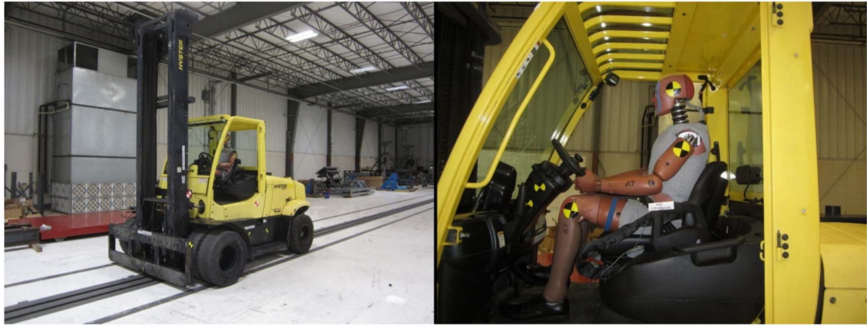
Fig. 1 Left pane: Class V Hyster lift truck with attachment removed; right pane: ATD positioning for test.
