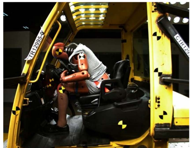
Fig. 5 ATD Head contact with a steering wheel in sled test
