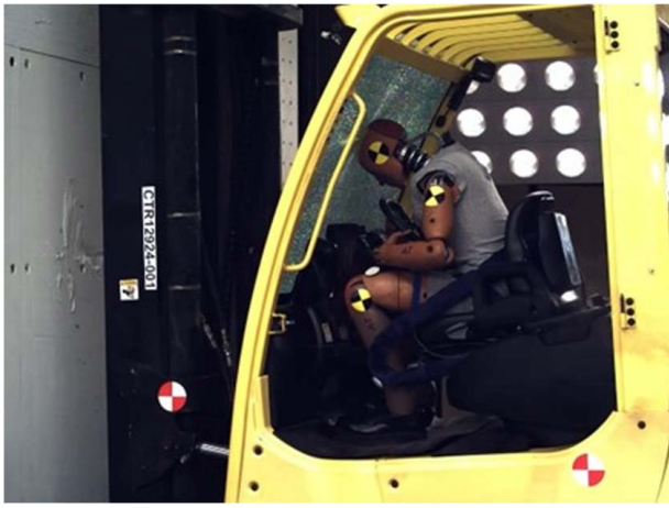
Fig. 3 ATD Head contact with windshield in the barrier test
