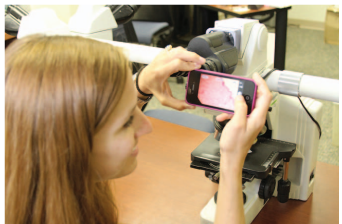
Holding the smart phone steady, the view beneath the microscope lens will fill the screen and an image can be captured.
