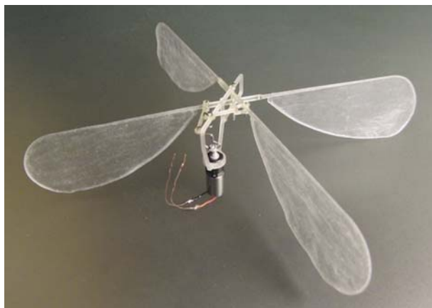
Figure 1. 3D-printed elements of flapping-hovering insect.
