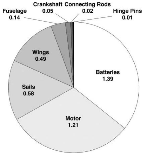
Figure 15. Breakdown of total mass (3.89 g).
