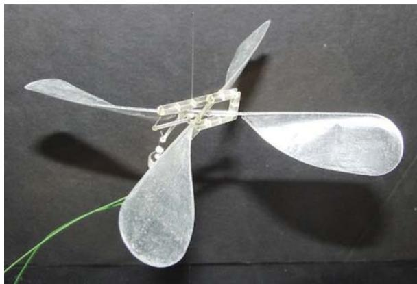
Figure 10. Wing deflection in a tethered flight test.
