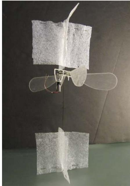
Figure 16. Final design with sails for passive stability.
