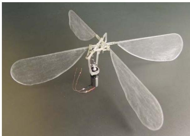
Figure 1. 3D-printed elements of flapping-hovering insect.
