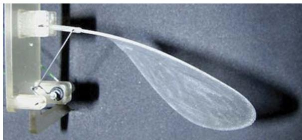
Figure 7. Flash photo showing deflection while flapping.
