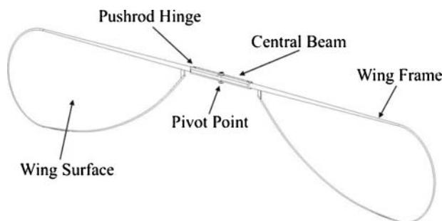
Figure 3. Parts of the one-piece printed wing.
