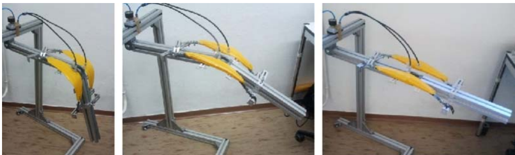
Figure 3. Biomechanical test bed simulating the knee joint, thigh, and shank. The knee joint is supported by a pair of feedback-controlled tensairity actuators. The picture shows a knee-joint extension sequence (left to right).
