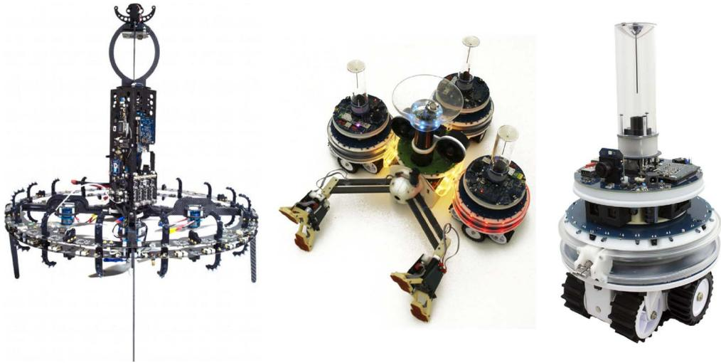
Figure 7. Swarmanoid eye-bot (left), hand-bot being carried by three foot-bots (center), and foot-bot (right). Courtesy of Marco Dorigo.
